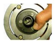
2. Place armature on top of shaft centering armature nut into compressor shaft.
