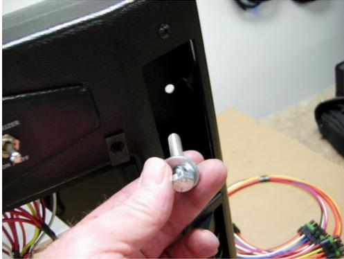
There are 4 holes (one in each corner) that will align with the unit, make sure the blower outlet is to the side of the switches of the console. Use 5/16 - 18 bolts with a flat washer(not provided), size accordingly to your roof thickness. You may need to seal the discharge area with foam to direct air into console
