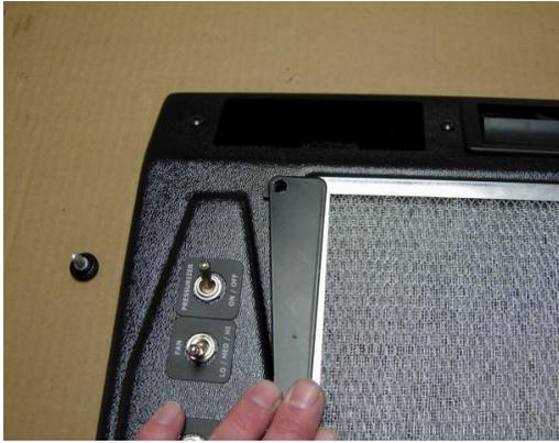
Align the filter hold down piece and fasten with thumb screws. An added benefit is this filter is easy to remove and can be rinsed with a garden hose for cleaning.
