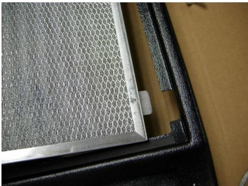
Reinstall the filter, make sure the tabs are to the bottom and are inserted into the slots in the console.
