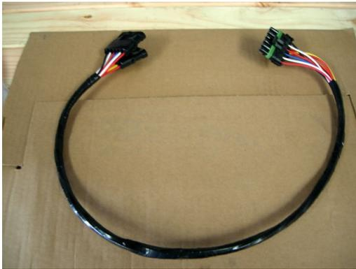
Reach up into the return air side of the unit on the roof and pull down the wire pigtail. If it will reach, plug it directly into the console. If it is short we have added an extension that can only be installed in one direction.
