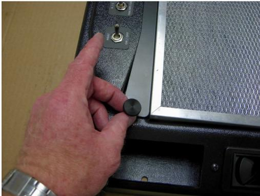
Remove the two thumb screws and the retaining metal hold down – then the filter will slide out of the plastic, there are tabs in the filter opposite of the thumb screws.
