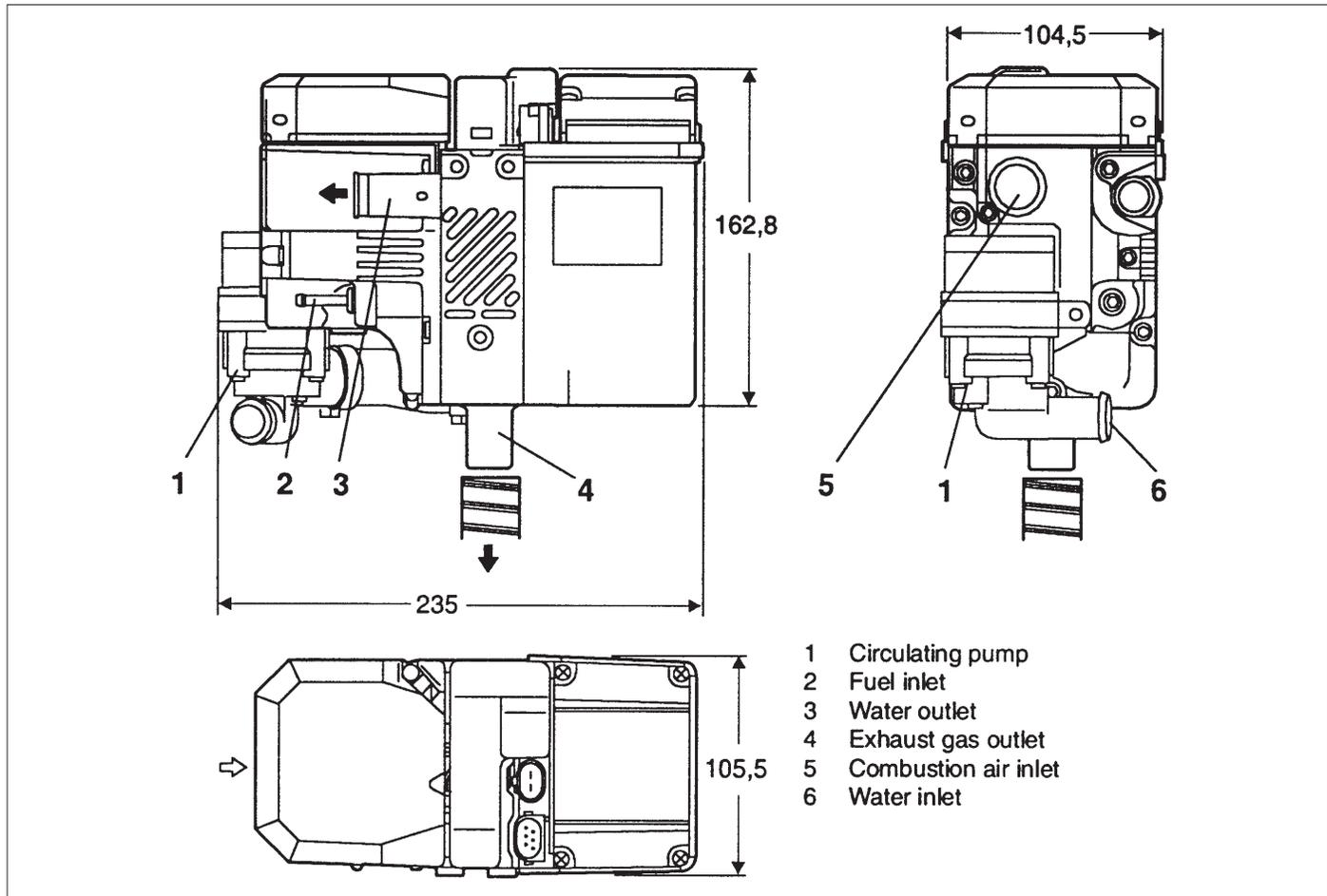
Fig. 301: Heater Dimensions
