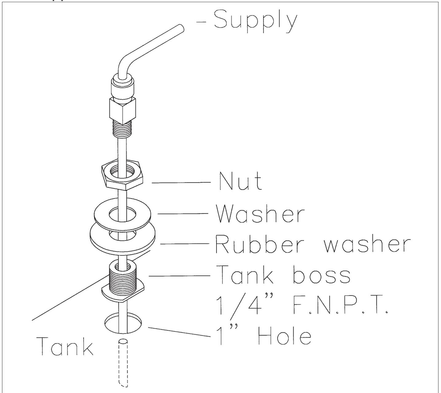
Fig. 406: Fuel Standpipe
