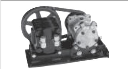
**Simple and straightforward, the hydraulic motor is connected to this compressor by the drive belt. Controlling the oil flow allows compressor regulation independent of engine speed.**
