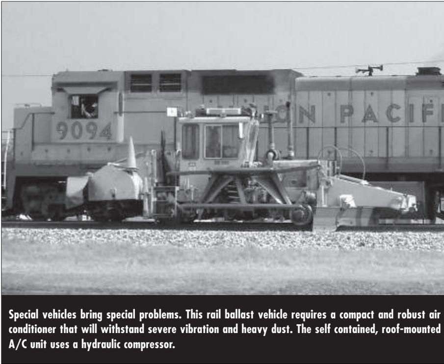
**Special vehicles bring special problems. This rail ballast vehicle requires a compact and robust air conditioner that will withstand severe vibration and heavy dust. The self contained, roof-mounted A/C unit uses a hydraulic compressor.**
