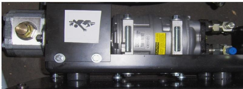
AN OEM APPLICATION FEATURING A TM-21 COMPRESSOR MATED WITH A HIGH PRESSURE MOTOR
