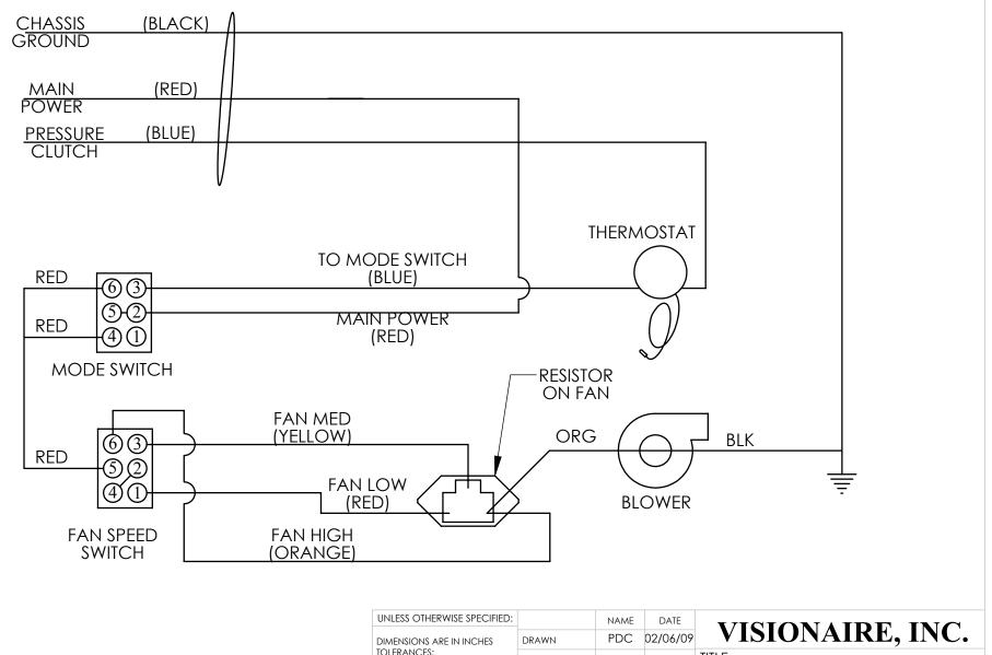
4050 A/C HEAT AND 4050 A/C ONLY WALL OR CEILING MOUNT EVAPORATOR
